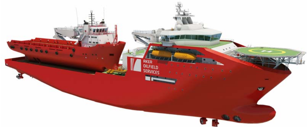
Illustration showing AKOFS OSCV 06 with modern PSV (84 x 19 m) on back deck
